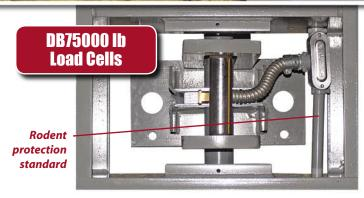
The EPR-LF+ Plus comes with 75,000-lb heavy-capacity, double-ended shear beam stainless steel load cells.
